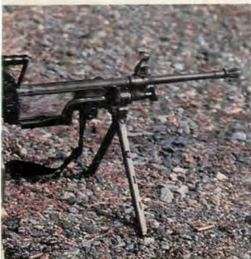
Deadly accuracy from reclining bipod fire. M249 in full-auto with 200-round plastic assault pack.
